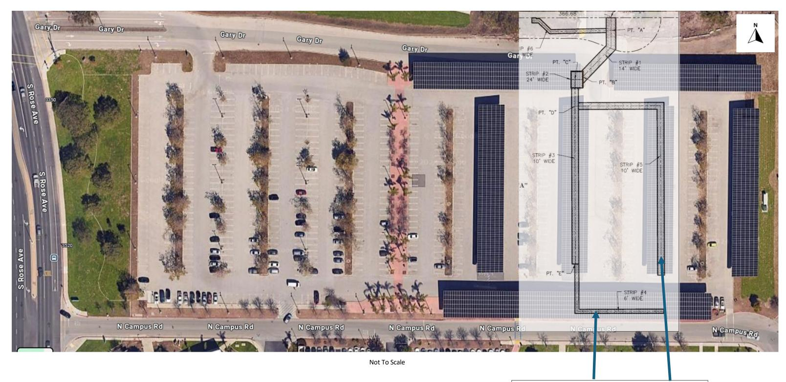
Easement "strips" are ground level underneath of the solar canopies.
